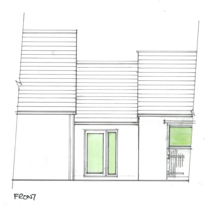
REMOVAL OF CONSERVATORY, CONSTRUCT FAMILY ROOM AND NEW RAISED ROOF AREA. COVERED YARD AREA FOR PORCH, WC AND BOOT/WET ROOM
