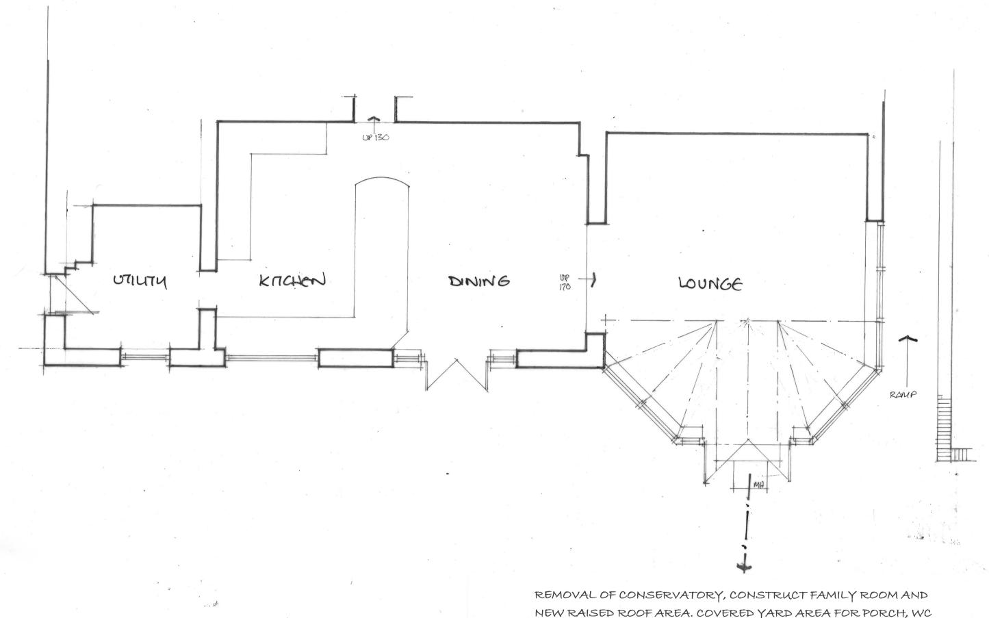
REMOVAL OF CONSERVATORY, CONSTRUCT FAMILY ROOM AND NEW RAISED ROOF AREA. COVERED YARD AREA FOR PORCH, WC AND BOOT/WET ROOM
