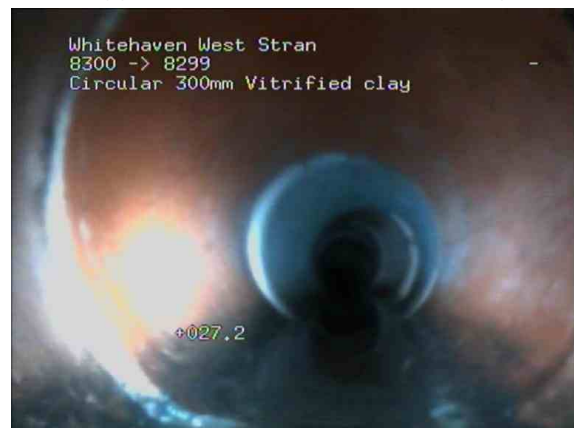
8300X_7e689ab5-758e-4139-a4b1-d54a4769d5c1_20210127 _091117_727.jpg, 00:07:11, 27.20 m Open joint, medium, start
