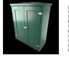
GRP ENCLOSURE DETAILS: 1400mm W x 660 D x REMOVABLE FLOOR 18mm PLY BACKBOARD HI/LOW VENTILATION IP65 MIN INTERNAL LIGHTING LOCK TO MATCH HOSPITAL STANDARD
