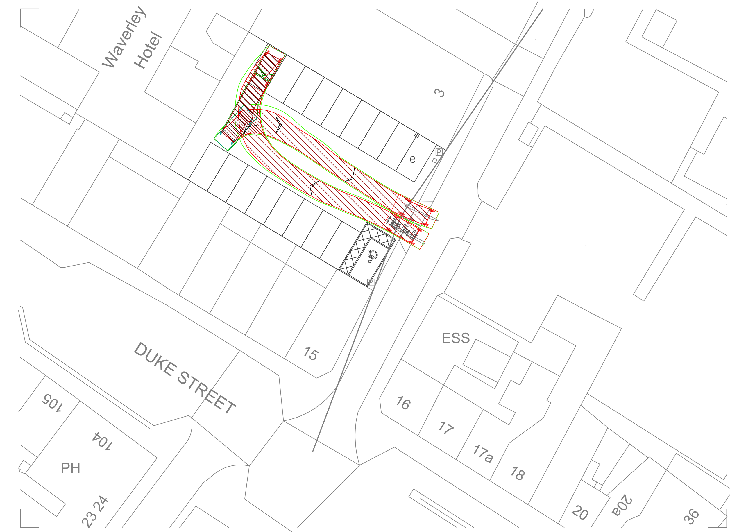
Vehicle Tracking Plan – Bay 2 Scale 1:250
