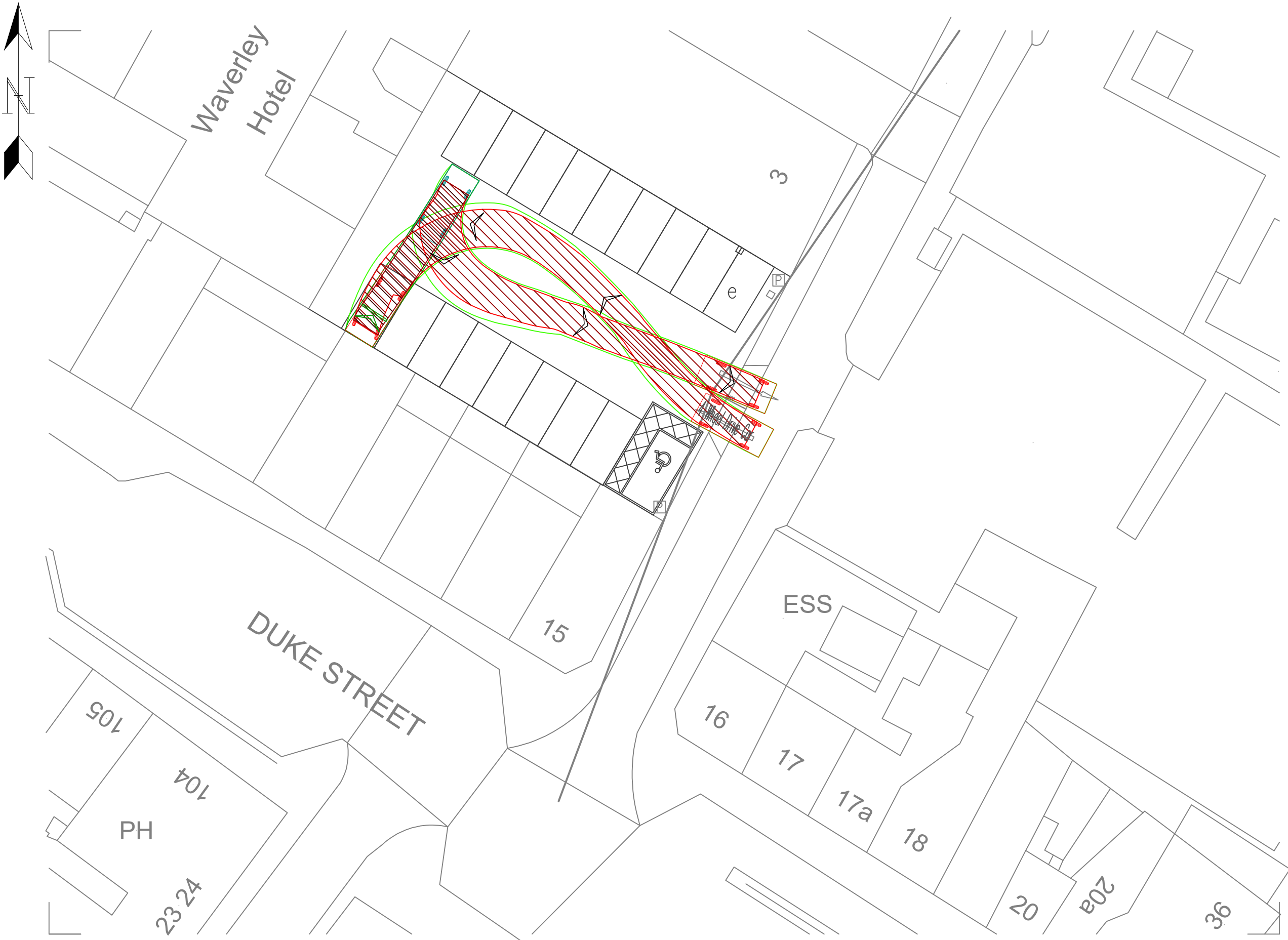
Vehicle Tracking Plan – Bay 1 Scale 1:250
