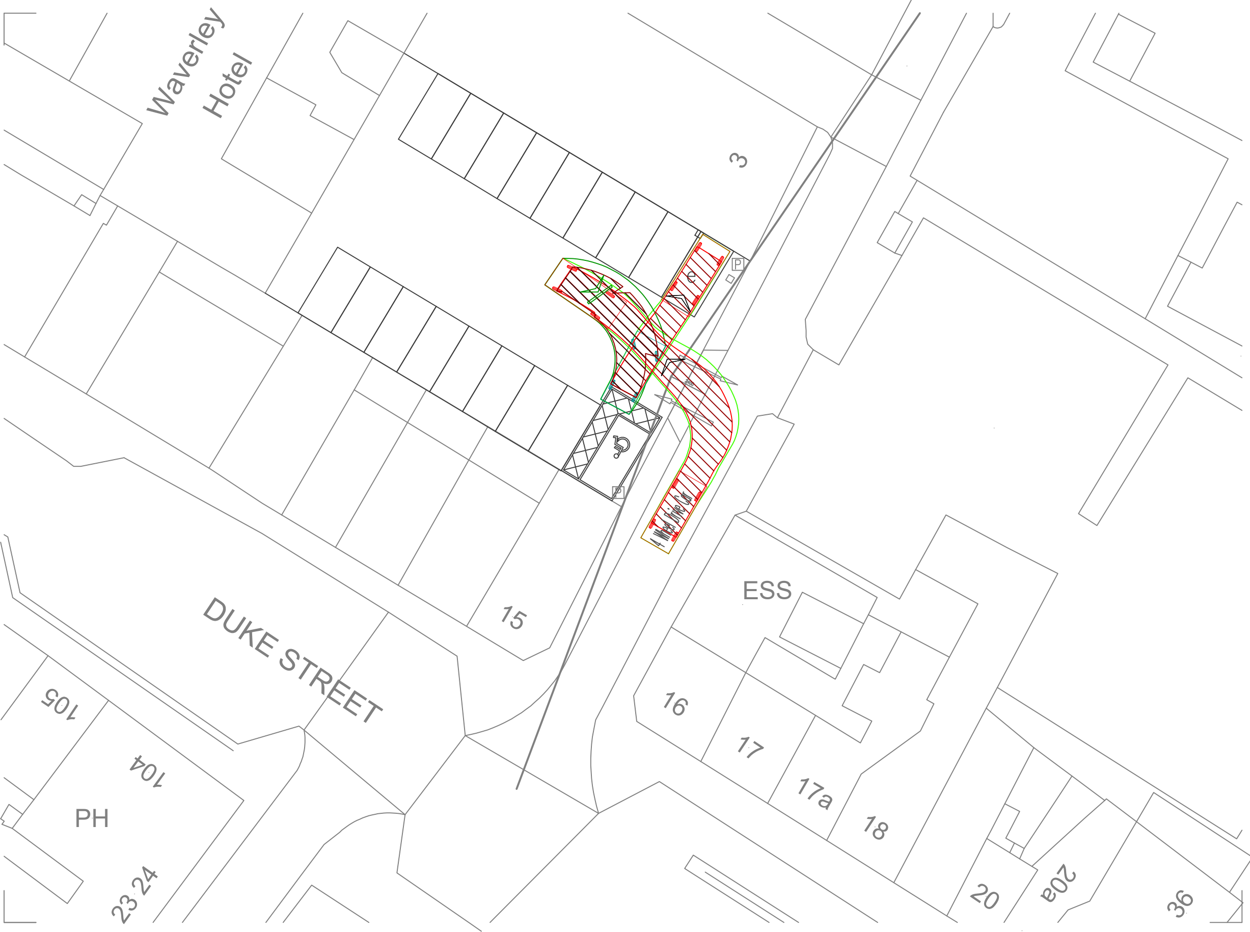
Vehicle Tracking Plan – Bay 3 Scale 1:250
