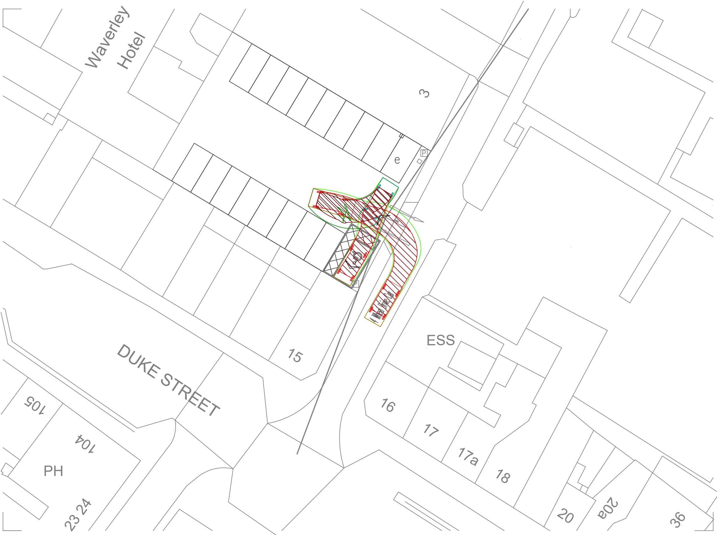
Vehicle Tracking Plan – Bay 4 Scale 1:250
