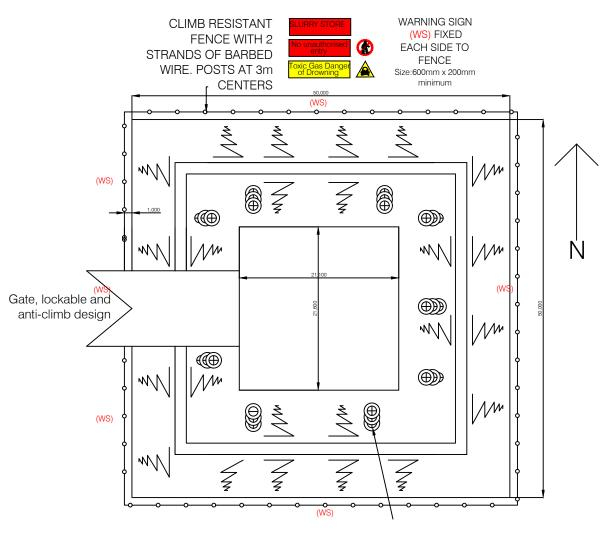
TYRES FIXED SECURELY TO THE TOP OF BANK AT INTERVALS OF 15m (MIN) TO FORM A METHOD OF ASSISTANCE TO CLIMB FROM LAGOON IN THE EVENT OF FALLING IN
