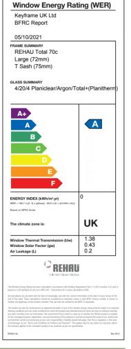
This Window Energy Rating has been calculated in accordance with Building Regulations Part L1b 2010 section 4.22 and is based on a UK standard window (1230mm wide x 1480mm high) as set out in BR 443 – Conventions for U value calculations, BRE 2006.
