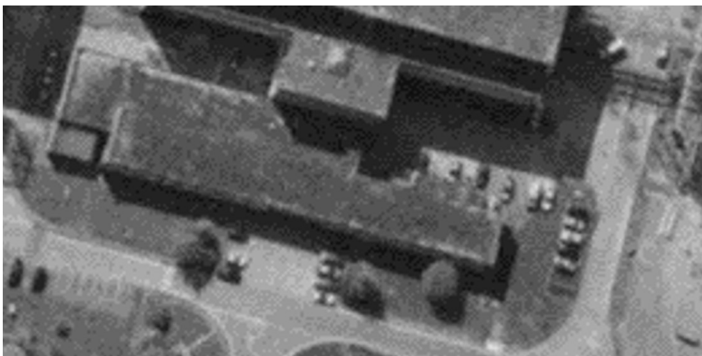
Figure 4 – Aerial photograph of the CHAB in 1998 showing the extended changeroom at the south-east end and the new kitchen extension at the north end of the west wall.
