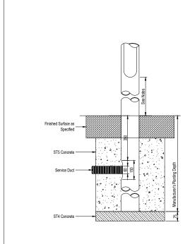
All dimensions are in millimetres and are the minimum requirement.
