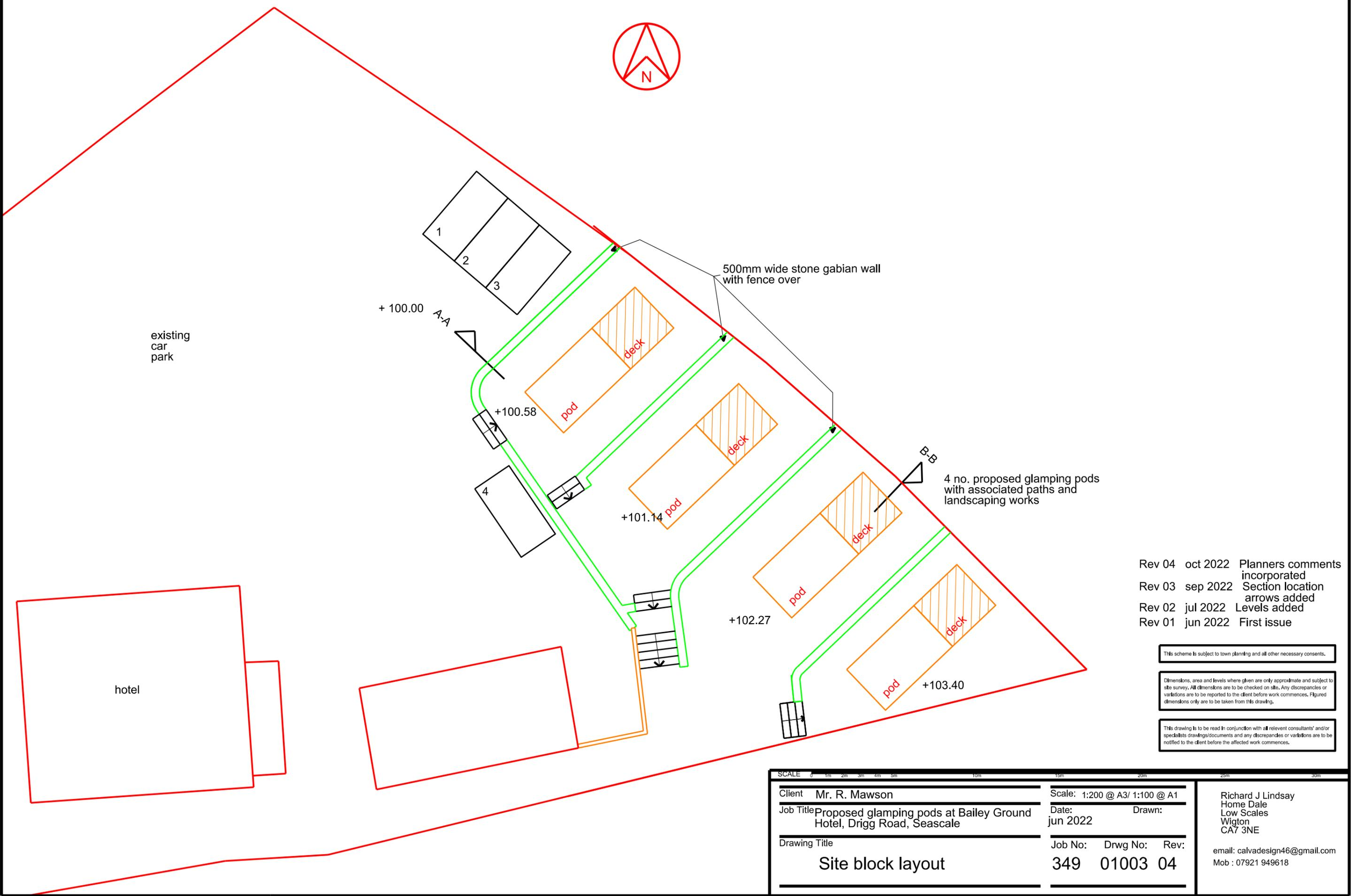
500mm wide stone gabion wall with fence over
