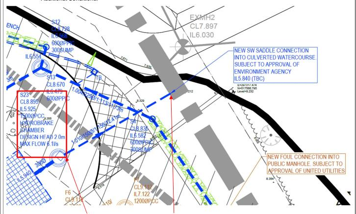
Connection to be made from S23 to existing 1700mm brick culverted watercourse.
