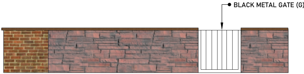
900 HIGH WALL, SANDSTONE TO FRONTAGE OF PLOTS 1,2,3, BRICK ELSE WHERE
