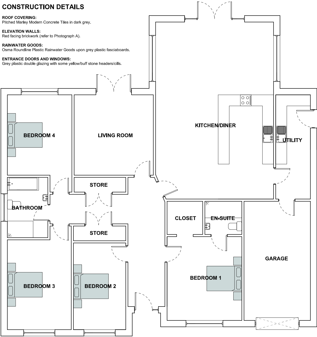
GROUND FLOOR PLAN SCALE 1:100
