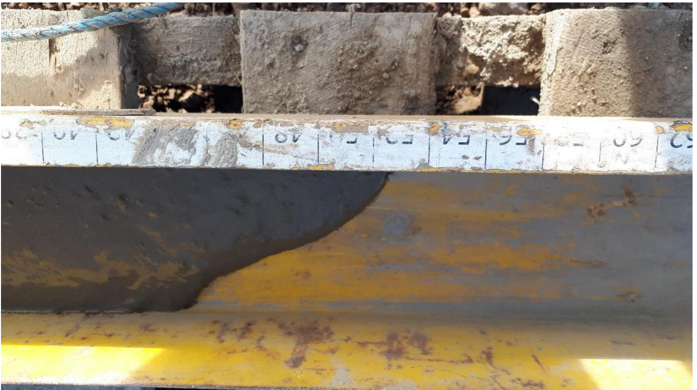
Photograph 6: Flow test at approximately 450mm.
