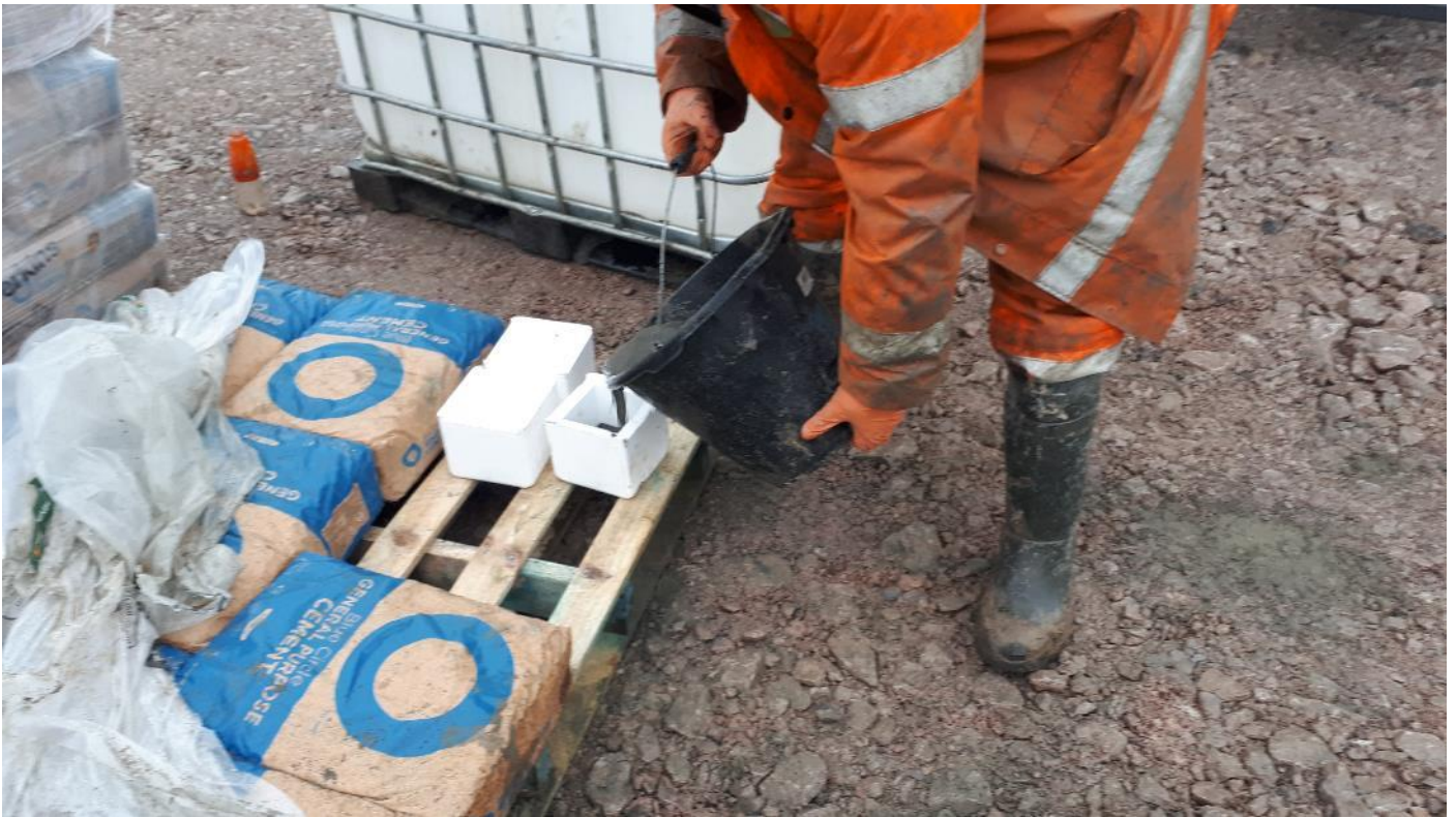
Photograph 7: Set of three grout cubes being cast.
