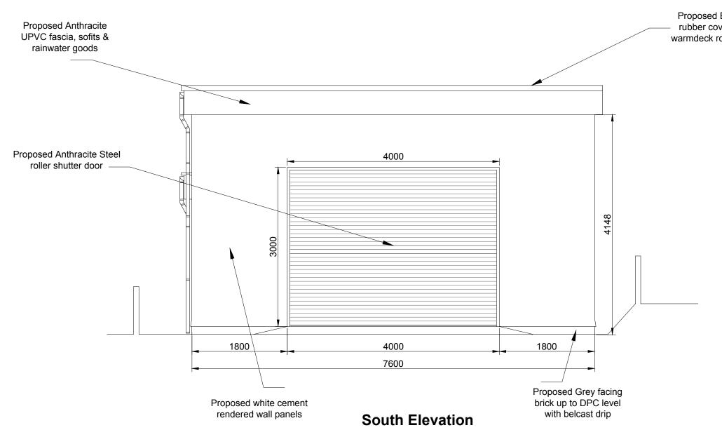
Proposed Black Firestone — rubber cover 150mm PIR warmdeck roofing membrane
