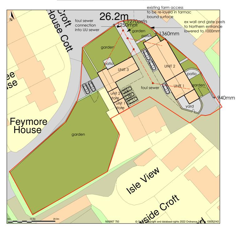
Block Plan shows area bounded by: 299027.29, 507459.02 299117.29, 507549.02 (at a scale of 1:500), OSGridRef: NX9907 750. The representation of a road, track or path is no evidence of a right of way. The representation of features as lines is no evidence of a property boundary
