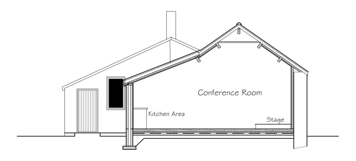
SECTION A-A AS PROPOSED (Central Truss Omitted for Clarity).
