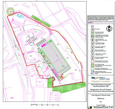
Retained Trees - Protective barriers to be erected around all retained trees in the position indicated by the blue line on the Tree Protection Plan prior to any works on site. Signs should also be attached stating that the area is a protected zone and should not be entered.
