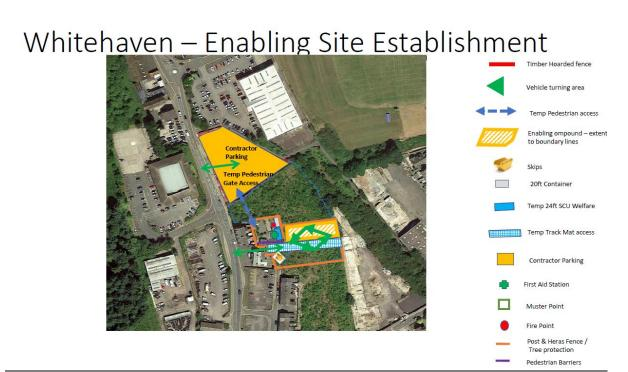
PROPOSED CONSTRUCTION WORKS - ENABLING SITE ESTABLISHMENT DRAWING
