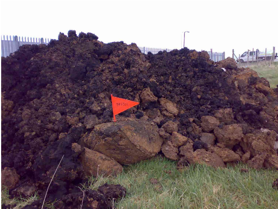
Plate 13 – Spoil of TP731E. Black soft clay had a thickness of about 1m at this location.
