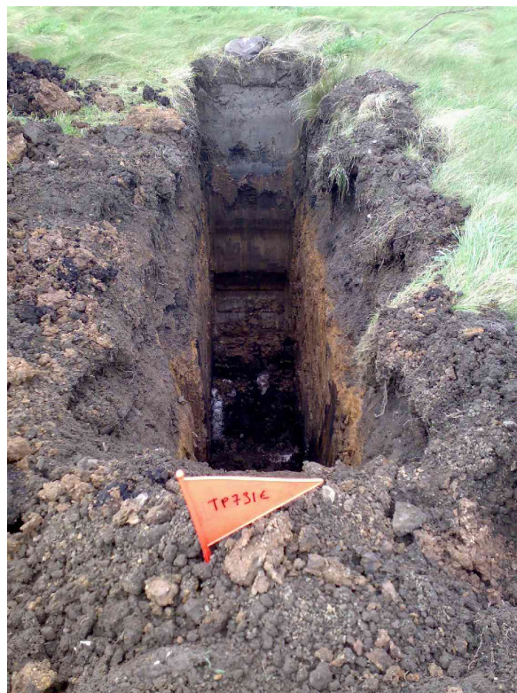
Plate 12 – TP731E. Brown gravelly clayey silt overlays brown-orange gravelly clay followed by black clay at about 1.9m bgl. Grey limestone was encountered at base of this trial pit (terminated at 2.6m bgl).
