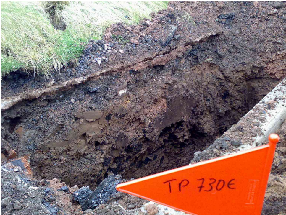
Plate 9 – TP730E covered with tarmac hardstanding underlain by hardcore fill material followed by dark brown sandy clay.
