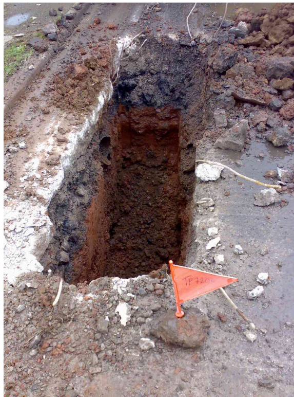
Plate 7 – TP720E Trial Pit is covered with concrete hardstanding overlaying hardcore fill material, followed by red-brown gravelly clay.
