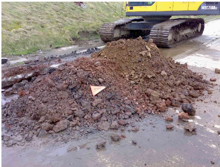
Plate 8 – Spoil of TP720E. Yellow brown limestone underlies red-brown clay (excavation terminated at 1.9m bgl).
