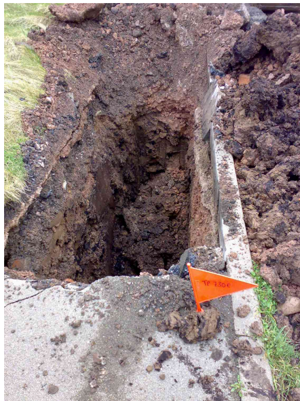
Plate 10 – TP730E. Brown sandy clay overlying pale grey-pink limestone (excavation terminated at 1.9m bgl).
