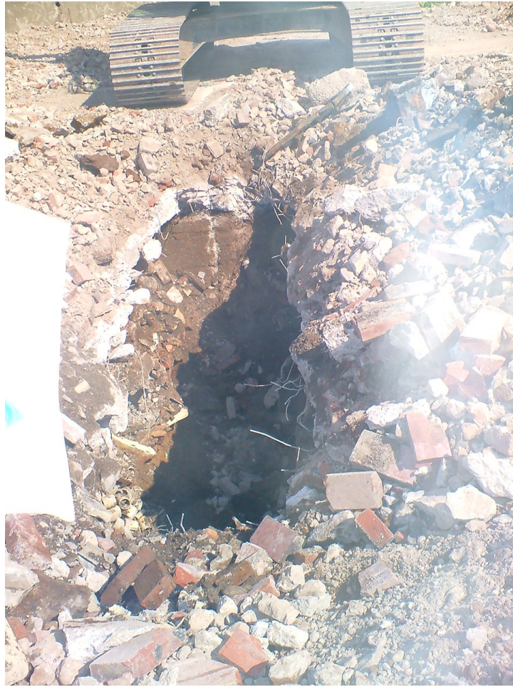
TP656B – 2.5m of loose Fill Material
