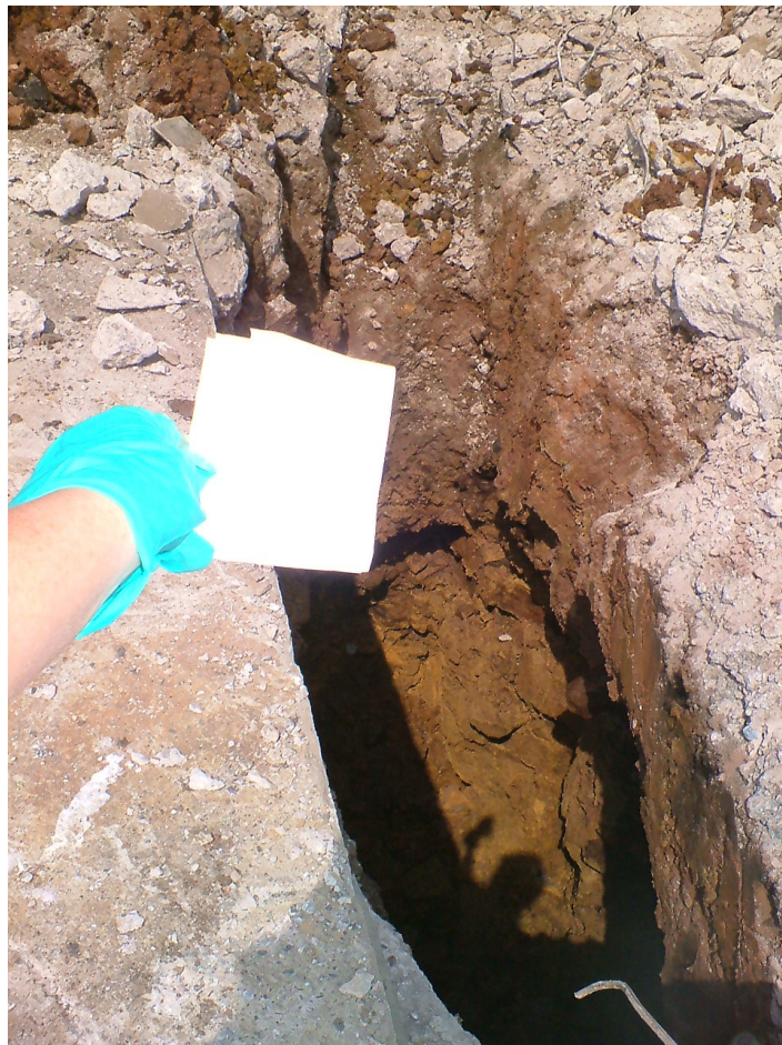
TP666B – yellow sandstone bedrock visible at base of trial pit
