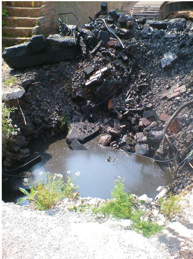
TP654B – black, perched ground water with strong chemical odour filled trial pit at 0.9m
