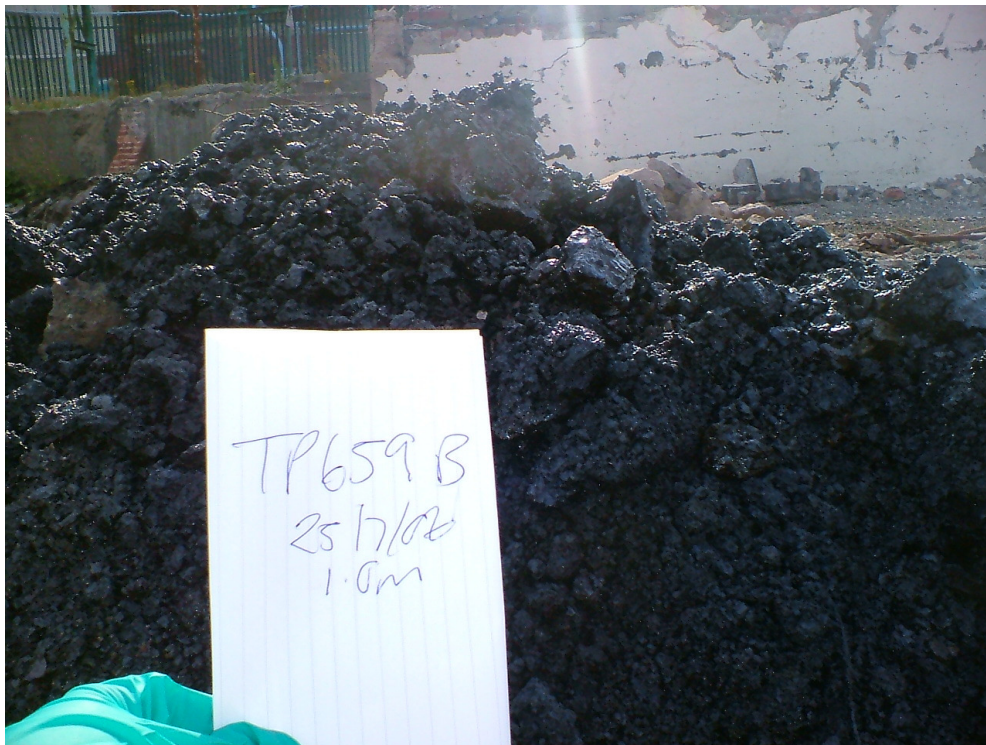
TP659B – black, oily staining of Made Ground
