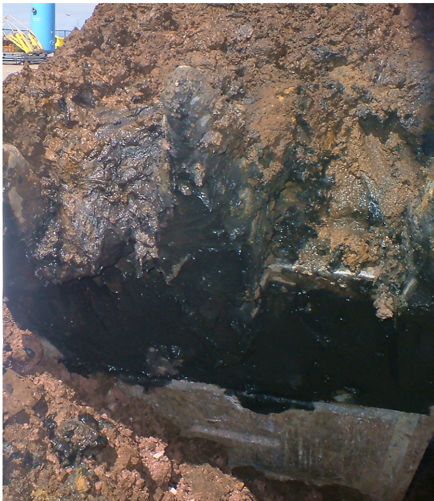
TP680B – black staining present at base Made Ground / top Drift
