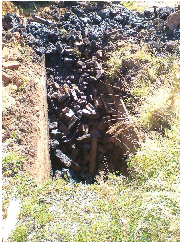
Photo 5 - TP615A – located in Plant Area, contaminated Fill Material between concrete foundations
