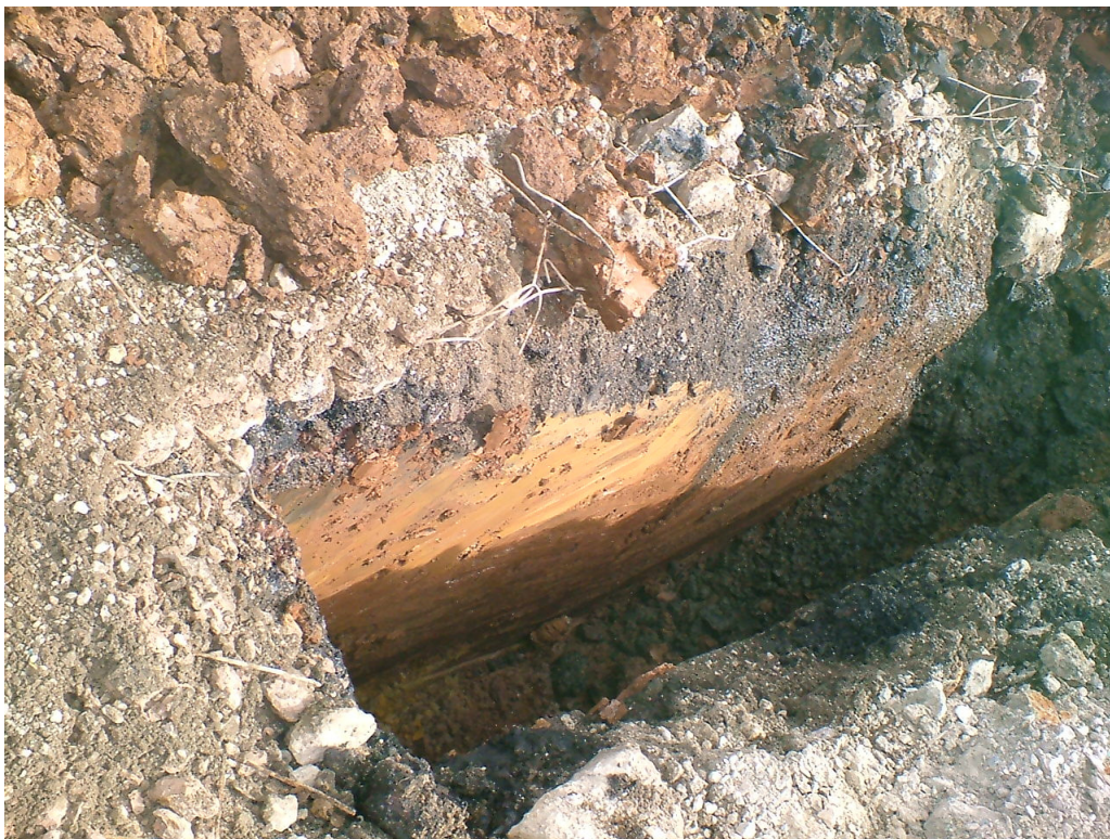
Photo 8 - TP628A – located in former Fatty Alcohol Plant, contaminated water running into trial pit through gravel Made Ground
