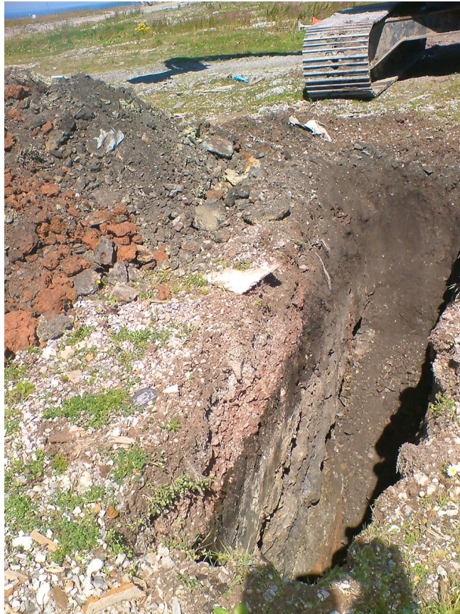
Photo 7 - TP622A – located in vicinity of former electrical substation, loose Fill Material
