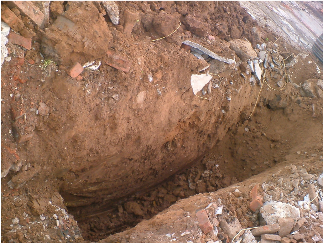
Photo 9 - TP630A – located in former Fatty Alcohol Plant, trial pit excavated into natural ground (Boulder Clay drift: firm red brown silt)
