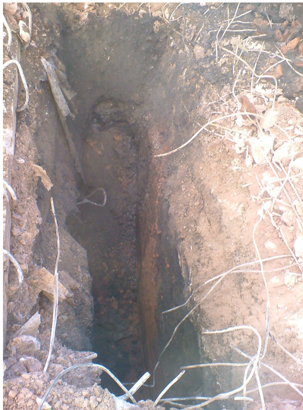
Photo 4 - TP607A – located in Cathedral Area, reinforced concrete and hardcore overlying Fill Material
