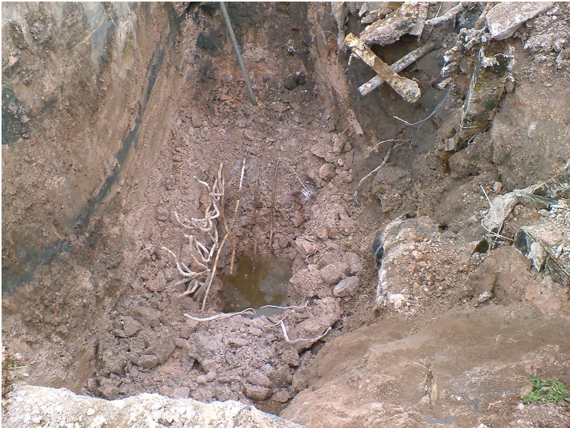
Trial Pit A108C- Steel reinforcement bars and standing water at the base of the trial pit
