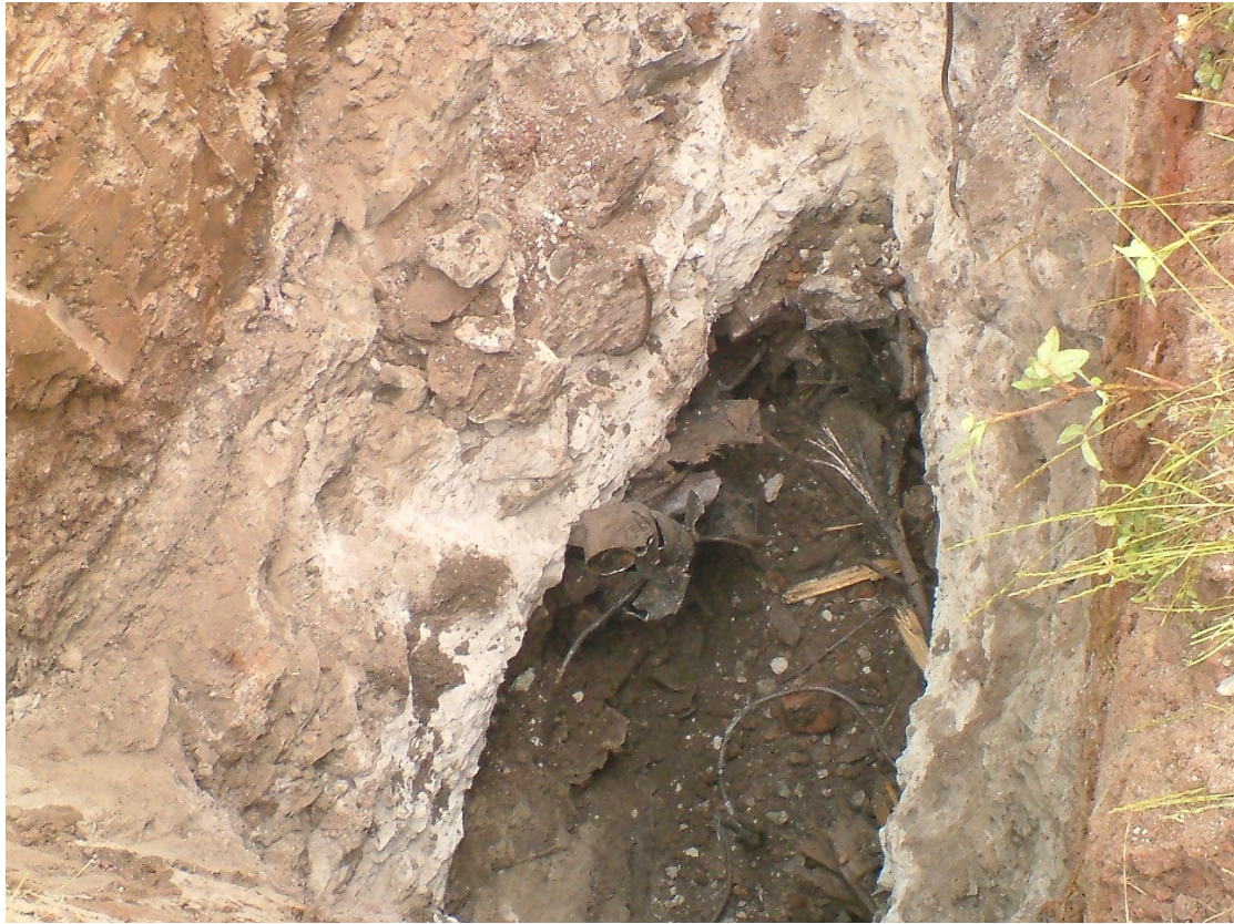
Trial Pit A109C (within Footprint of North Pond)- Significant thickness of concrete (1.3m thick)
