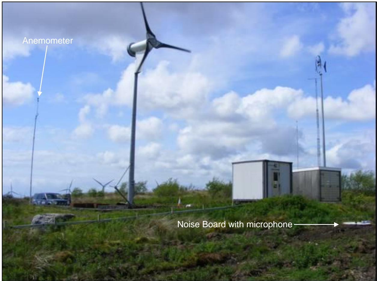
FIGURE 1 PHOTOGRAPH SHOWING ACOUSTIC TEST ARRANGEMENT
