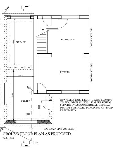
WALLS WALLS SHALL BE 300mm CAVITY CONSTRUCTION TO COMPRISE: BELOW DPC-100mm thk. BLOCKWORK INNER LEAF CELCON THERMOLITE SHIELD TYPE OR EQUAL AND APPROVED AND 100mm THK DENSE CONCRETE OUTER LEAF WITH WEAK MIX CAVITY FILL.WEAK MIX CAVITY FILL SHALL NOT BE WITHIN 225mm OF THE DPC AS PER DIAGRAM 9a OF APPROVED DOCUMENT C. ALLOW FOR HY-LOAD DPC BEDDED IN CEMENT MORTAR. DPC SHALL BE 150mm MIN ABOVE EXTERNAL GROUND LEVEL.
