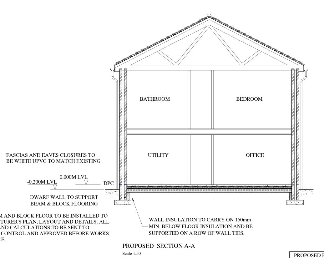
EXACT DETAILS OF FULL ROOF PLANS ALONG WITH MANUFACTURERS DESIGN CALCULATIONS DETAILS AND LAYOUT TO BE ISSUED TO BUILDING CONTROL BY ROOFING CONTRACTOR PRIOR TO WORKS BEING CARRIED OUT. EXACT DIMENSIONS SHALL BE ESTABLISHED ON SITE
