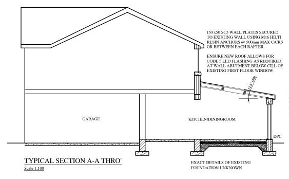
NEW ROOF TO HAVE 165mm MIN. INSULATION LAID BETWEEN RAFTERS TO ACHIEVE A MAXIMUM 'U' VALUE OF 0.18W/M<sup>2</sup>K CELOTEX XR4000, OR EQUAL AND APPROVED ALL INSTALLED TO
