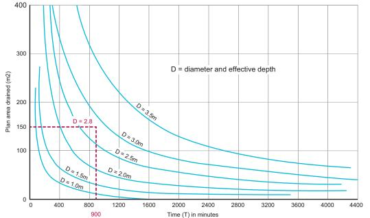
From the graph below, the diameter and effective depth of the soakaway (D) are both 2.8m.
