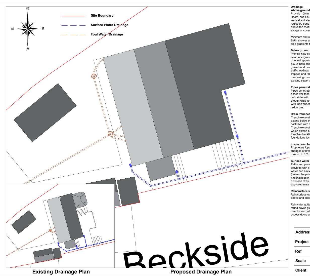
Provide 100 mm soil vent pipes to take waste pipes from Bathroom, Shower Room, and En-suite. Refer to drawing for location of s.v.ps. Drain invert to vertical soil stack to be min. 450 mm below lowest connection point (large radius 90 bend). Stacks to be ventilated at head of drain and terminated above the roof line, 900 mm above any opening within 3m, and finished with a cage or cover which does not restrict the flow of air.
