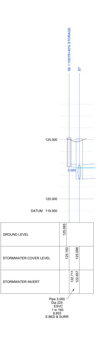
ALL COVER & INVERT LEVEL INFORMATION HAS BEEN TAKEN FROM AVAILABLE TOPOGRAPHICAL SURVEY DATA OR UNITED UTILITY RECORDS AND CCTV REPORT. EXISTING PUBLIC FOUL AND SURFACE WATER SEWERS ARE TO BE ABOVE GROUND PROBED, ROUTED AND INTERNALLY SURVEYED WITH ALL INFORMATION PASSED TO SITE INFRASTRUCTURE SERVICES LTD FOR REVIEW PRIOR TO COMMENCEMENT ON SITE
