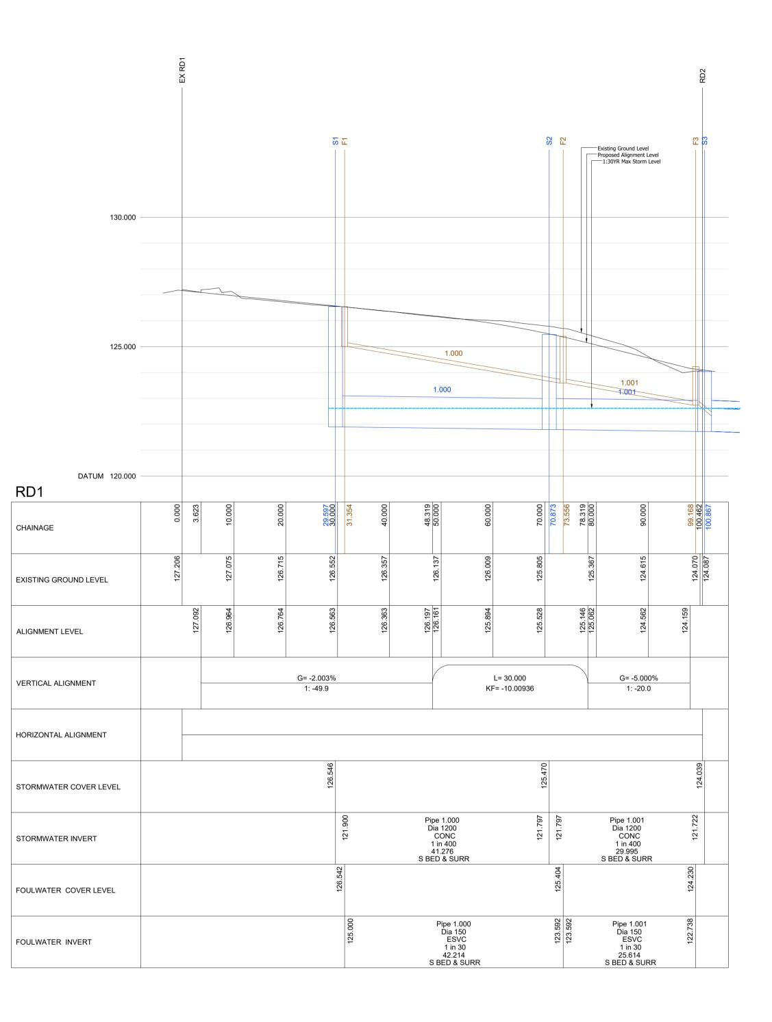
ALL COVER & INVERT LEVEL INFORMATION HAS BEEN TAKEN FROM AVAILABLE TOPOGRAPHICAL SURVEY DATA OR UNITED UTILITY RECORDS AND CCTV REPORT. EXISTING PUBLIC FOUL AND SURFACE WATER SEWERS ARE TO BE ABOVE GROUND PROBED, ROUTED AND INTERNALLY SURVEYED WITH ALL INFORMATION PASSED TO SITE INFRASTRUCTURE SERVICES LTD FOR REVIEW PRIOR TO COMMENCEMENT ON SITE
