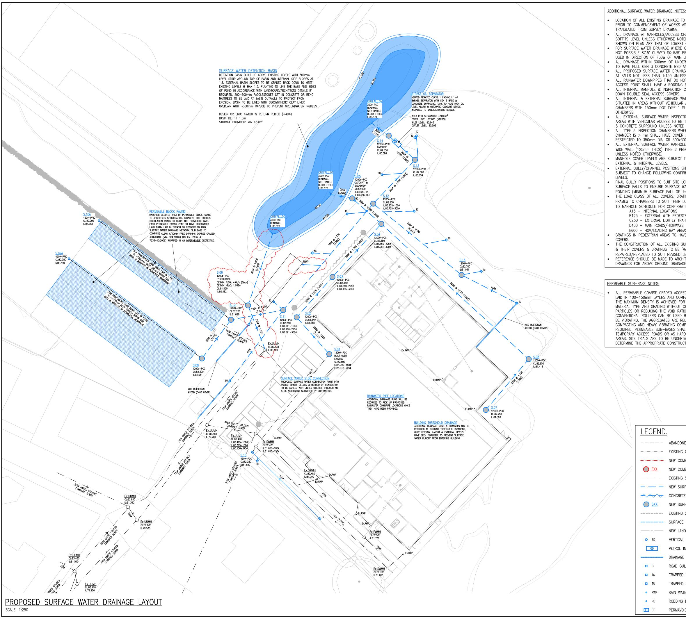
LOCATION OF ALL EXISTING DRAINAGE TO BE CONFIRMED ON SITE PRIOR TO COMMENCEMENT OF WORKS AS IT IS APPROXIMATELY TRANSLATED FROM SURVEY DRAWING. ALL DRAINAGE AT MANHOLES/ACCESS CHAMBERS TO CONNECT WITH SOFFITS LEVEL UNLESS OTHERWISE NOTED. MANHOLE INVERT LEVELS SHOWN ON PLAN ARE THAT OF LOWEST OUTGOING PIPE. FOR SURFACE WATER DRAINAGE WHERE OBLIQUE CONNECTIONS ARE NOT POSSIBLE 87.5° CURVED SQUARE BRANCH CONNECTIONS TO BE USED IN DIRECTION OF FLOW OF MAIN LINE.
