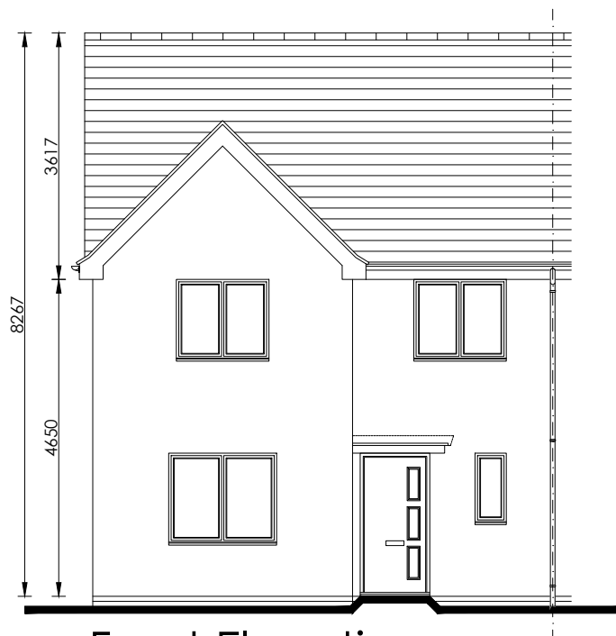
Front Elevation scale 1:100
