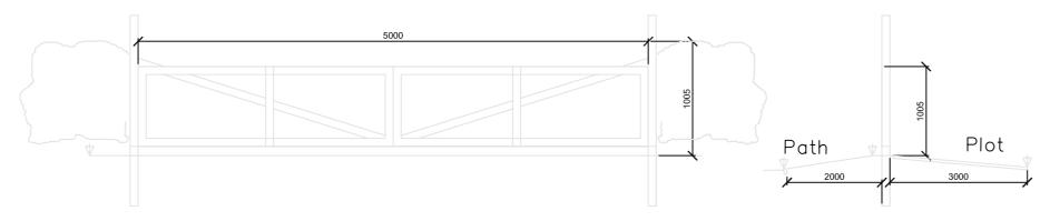
Terram BodPave 40 porous (Green) paving grids installed to manufacturers recommendations and details Ground falls away by 200mm over 3m Max hedge height 1.05m to ensure clear vision
