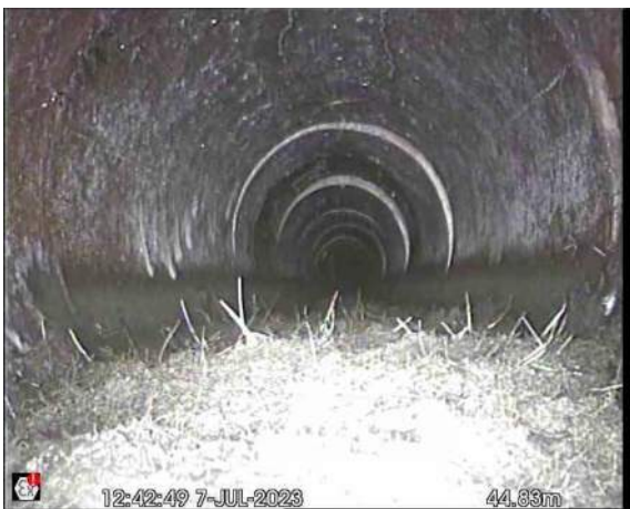
S1X_3c923e43-07ef-43e7-ab5b-b781b3bc5df2_20230712_153641_621.jpg, 00:03:05, 44.83 m Roots, mass, 25% cross-sectional area loss
