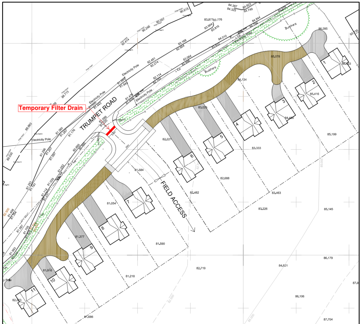
Figure 4.1 Location of temporary filter drain at site entrance
