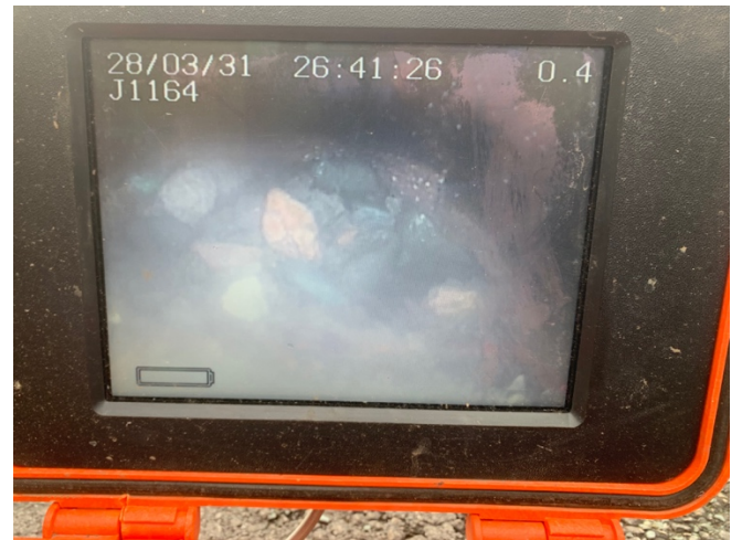
Fig 7. Outlet pipe blocked
