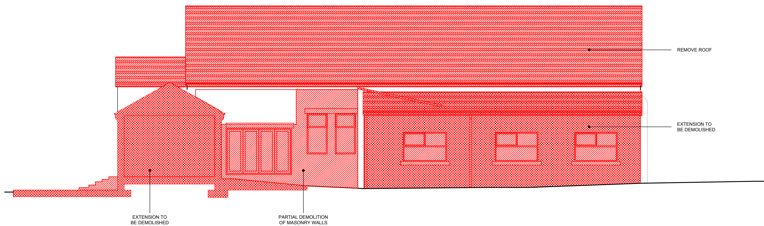
3 MILLWAY: Existing & Demolition South Elevation 1:100 @ A1
