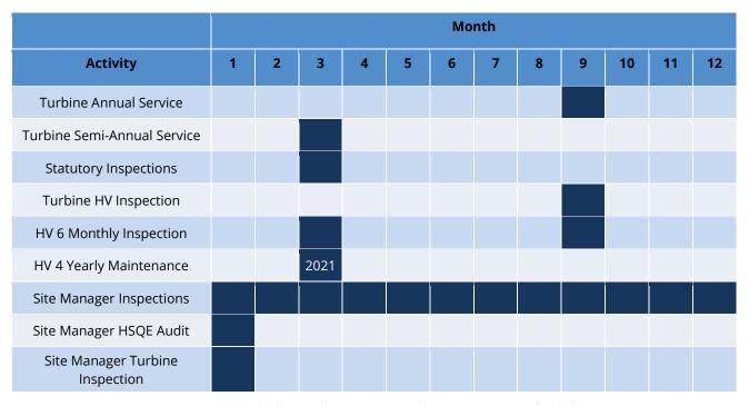
Figure 1: Typical Planned Inspection and Maintenance Schedule
