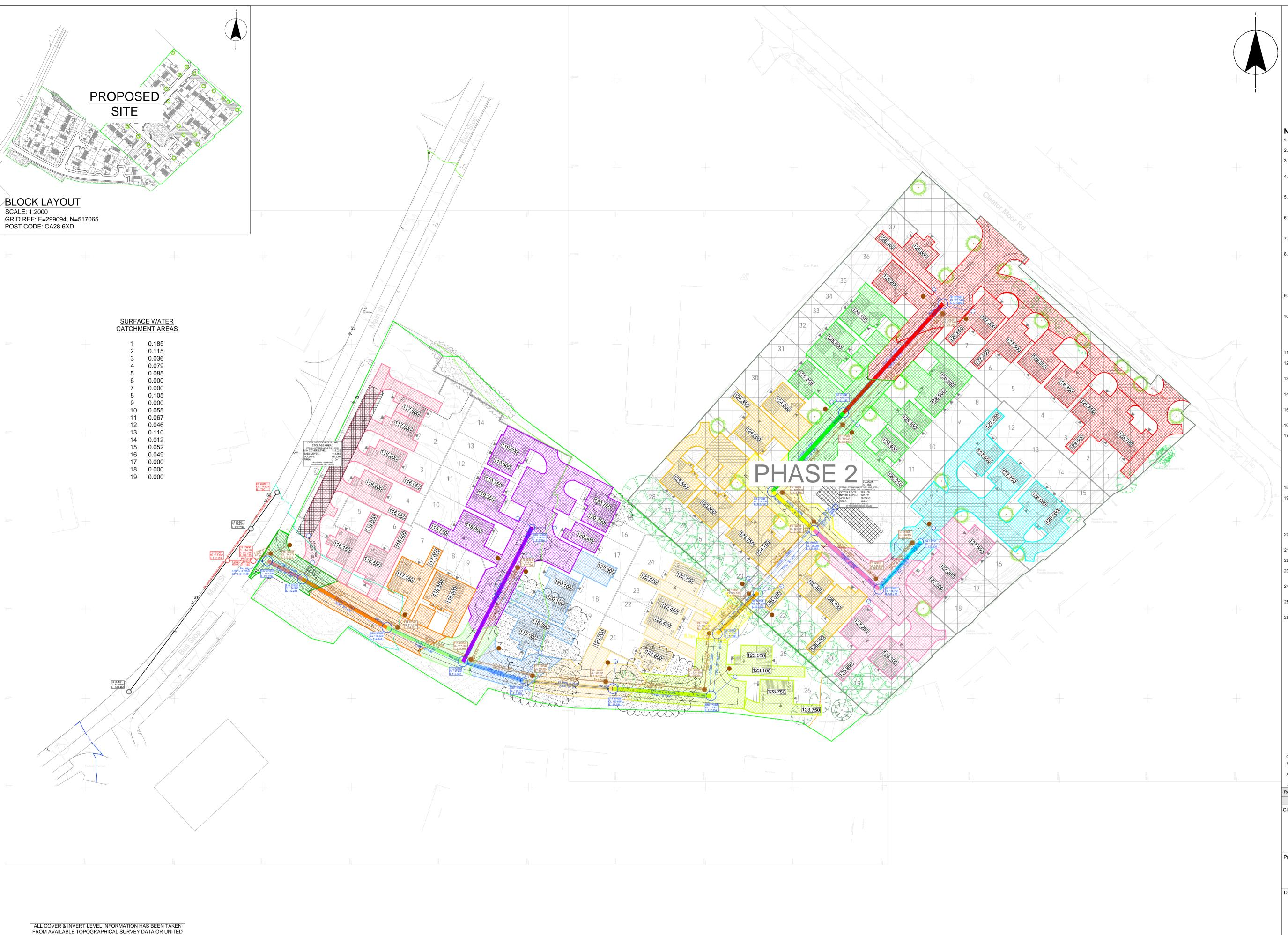
UTILITY RECORDS AND CCTV REPORT. EXISTING PUBLIC FOUL AND SURFACE WATER SEWERS ARE TO BE ABOVE GROUND PROBED, ROUTED AND INTERNALLY SURVEYED WITH ALL INFORMATION PASSED TO SITE INFRASTRUCTURE SERVICES LTD FOR REVIEW PRIOR TO COMMENCEMENT ON SITE
