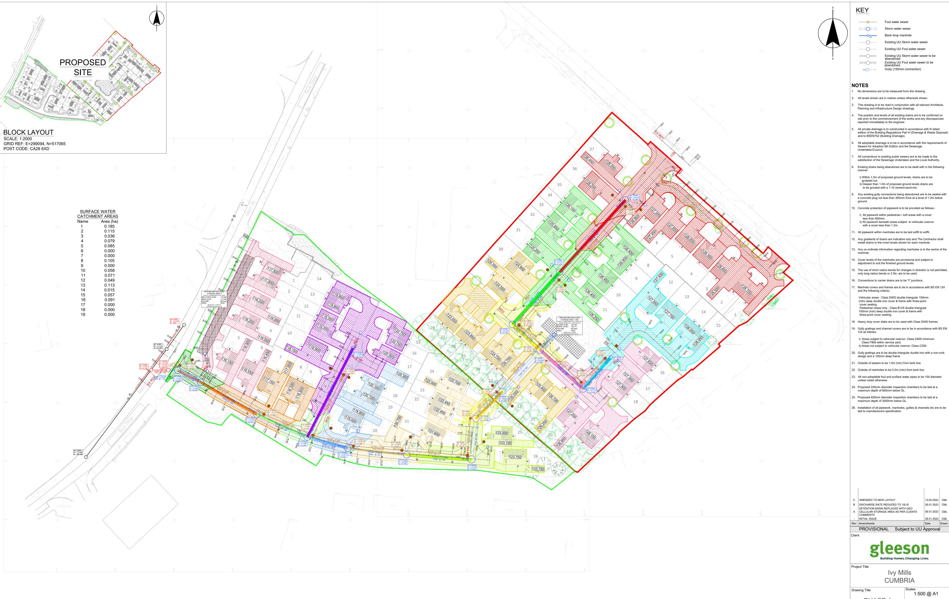
ALL COVER & INVERT LEVEL INFORMATION HAS BEEN TAKEN FROM AVAILABLE TOPOGRAPHICAL SURVEY DATA OR UNITED UTILITY RECORDS AND CCTV REPORT. EXISTING PUBLIC FOUL AND SURFACE WATER SEWERS ARE TO BE ABOVE GROUND PROBED, ROUTED AND INTERNALLY SURVEYED WITH ALL INFORMATION PASSED TO SITE INFRASTRUCTURE SERVICES LTD FOR REVIEW PRIOR TO COMMENCEMENT ON SITE
