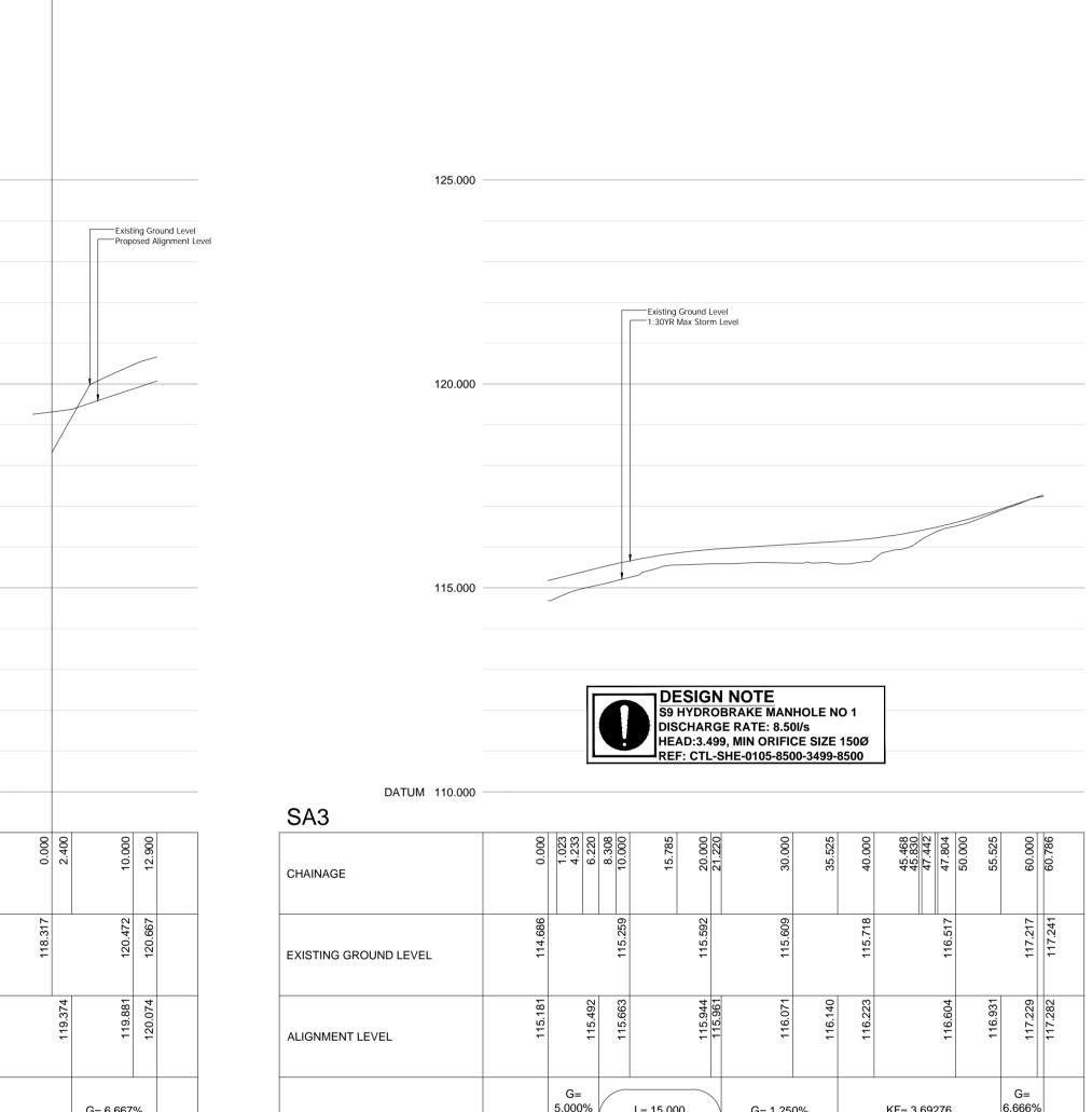
ALL COVER & INVERT LEVEL INFORMATION HAS BEEN TAKEN FROM AVAILABLE TOPOGRAPHICAL SURVEY DATA OR UNITED UTILITY RECORDS AND CCTV REPORT. EXISTING PUBLIC FOUL AND SURFACE WATER SEWERS ARE TO BE ABOVE GROUND PROBED, ROUTED AND INTERNALLY SURVEYED WITH ALL INFORMATION PASSED TO SITE INFRASTRUCTURE SERVICES LTD FOR REVIEW PRIOR TO COMMENCEMENT ON SITE
