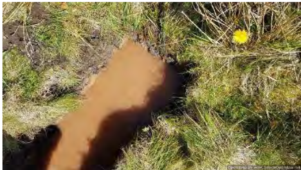
Trial Pit TP01 – Start of infiltration Test
