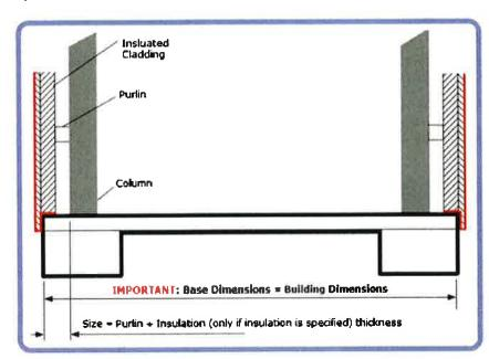
To ensure a weather we recommend seal creating a base that is raised off ground level by a minimum of 50mm to allow our cladding to overhang the base and promote water to run the away from structure. Our buildings can be erected to oversized bases/yards however this does introduce the need for an alternative method of creating a around the
