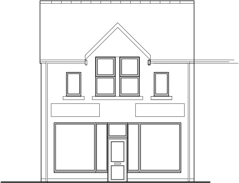
EXISTING FRONT ELEVATION timber door timber windows
