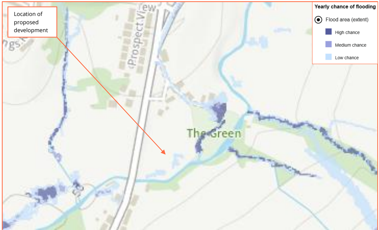
Figure 8: Extract from EA Risk of Flooding from Surface Water mapping – present day (Source: EA)
