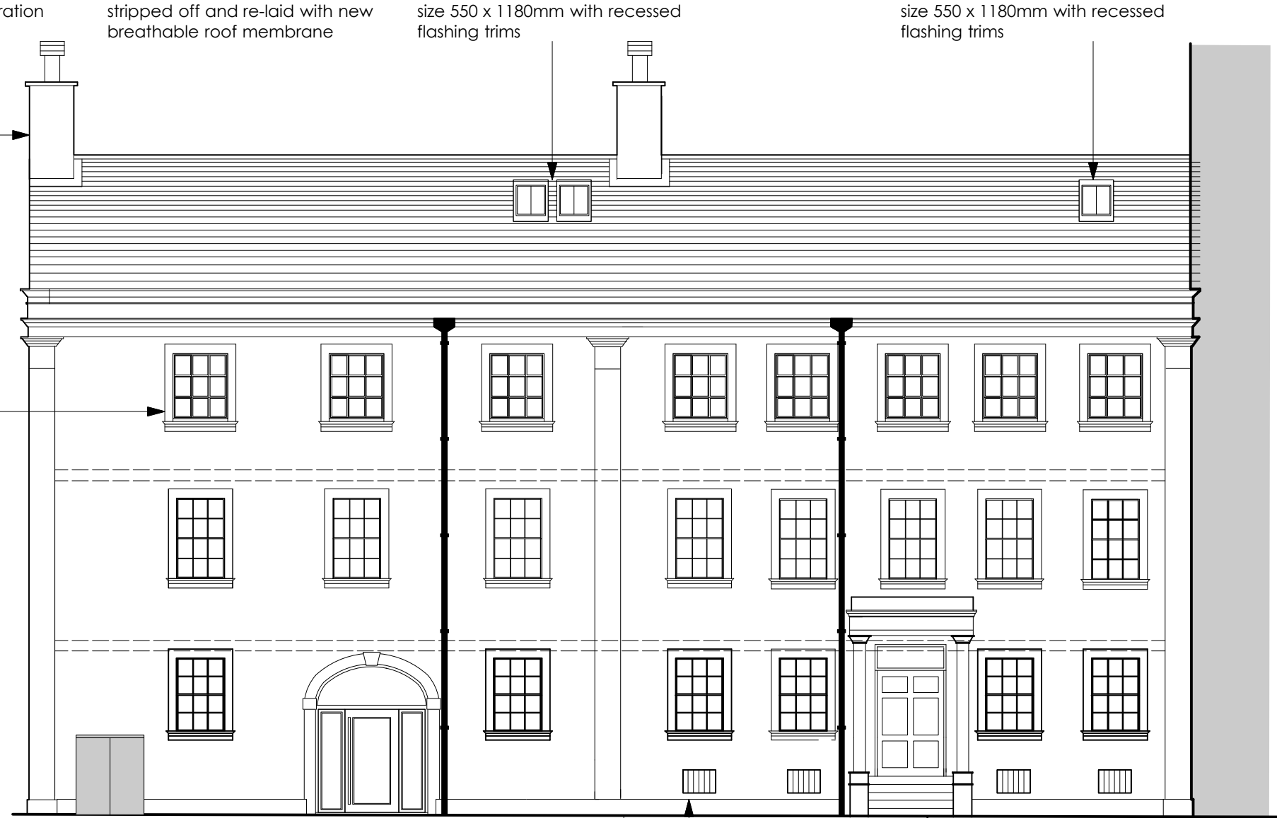
Front Elevation to Harbour new timber double glazed door screen - existing railing to side of ramp removed
