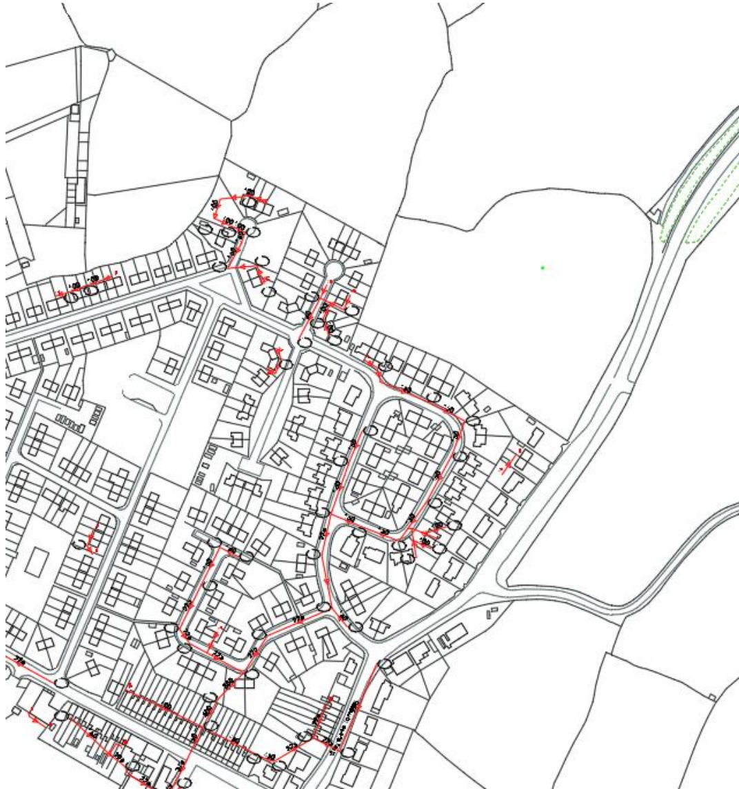
Figure 3.5.1 - Sewer Record Drawing.
