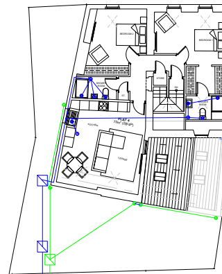
6 01_Second Floor Plumbing Plan
