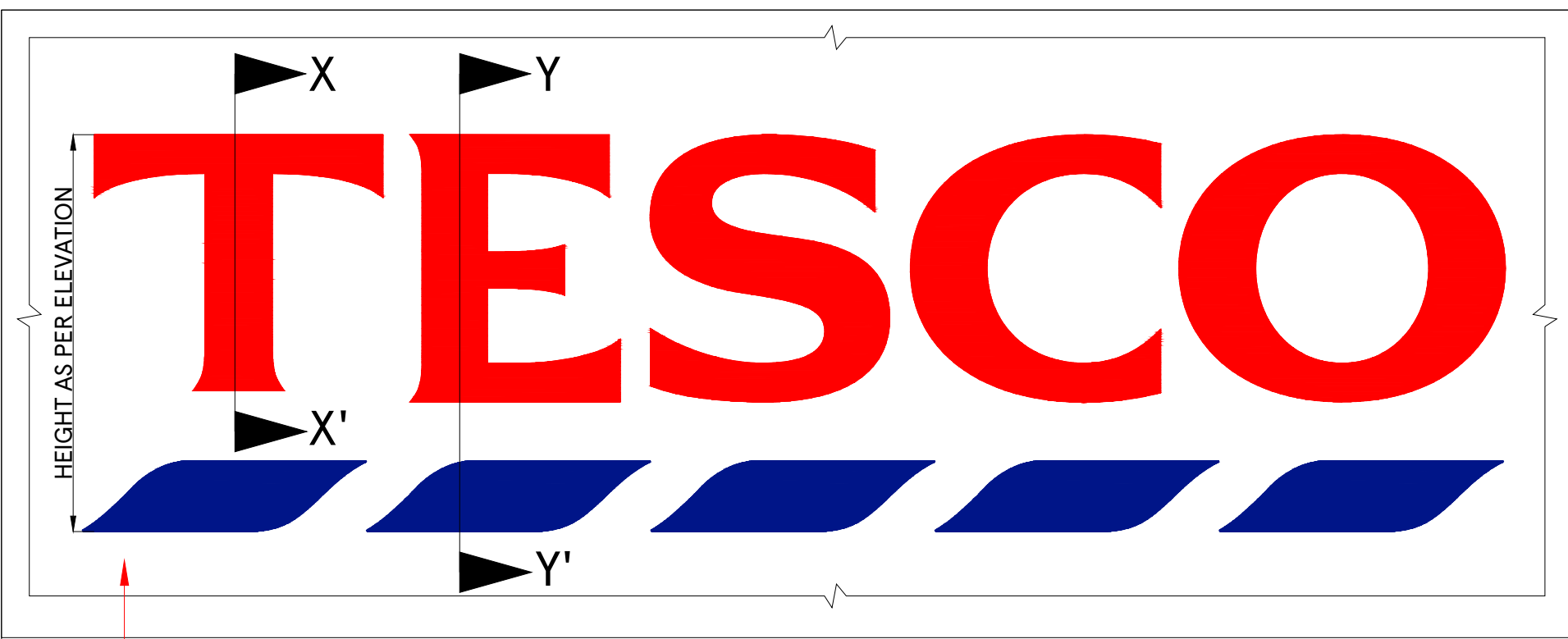
PART ELEVATION: Built-Up Acrylic Letters (internal illuminated) installed on 2mm Formed Aluminum Fascia Panel [Scale 1:20]
