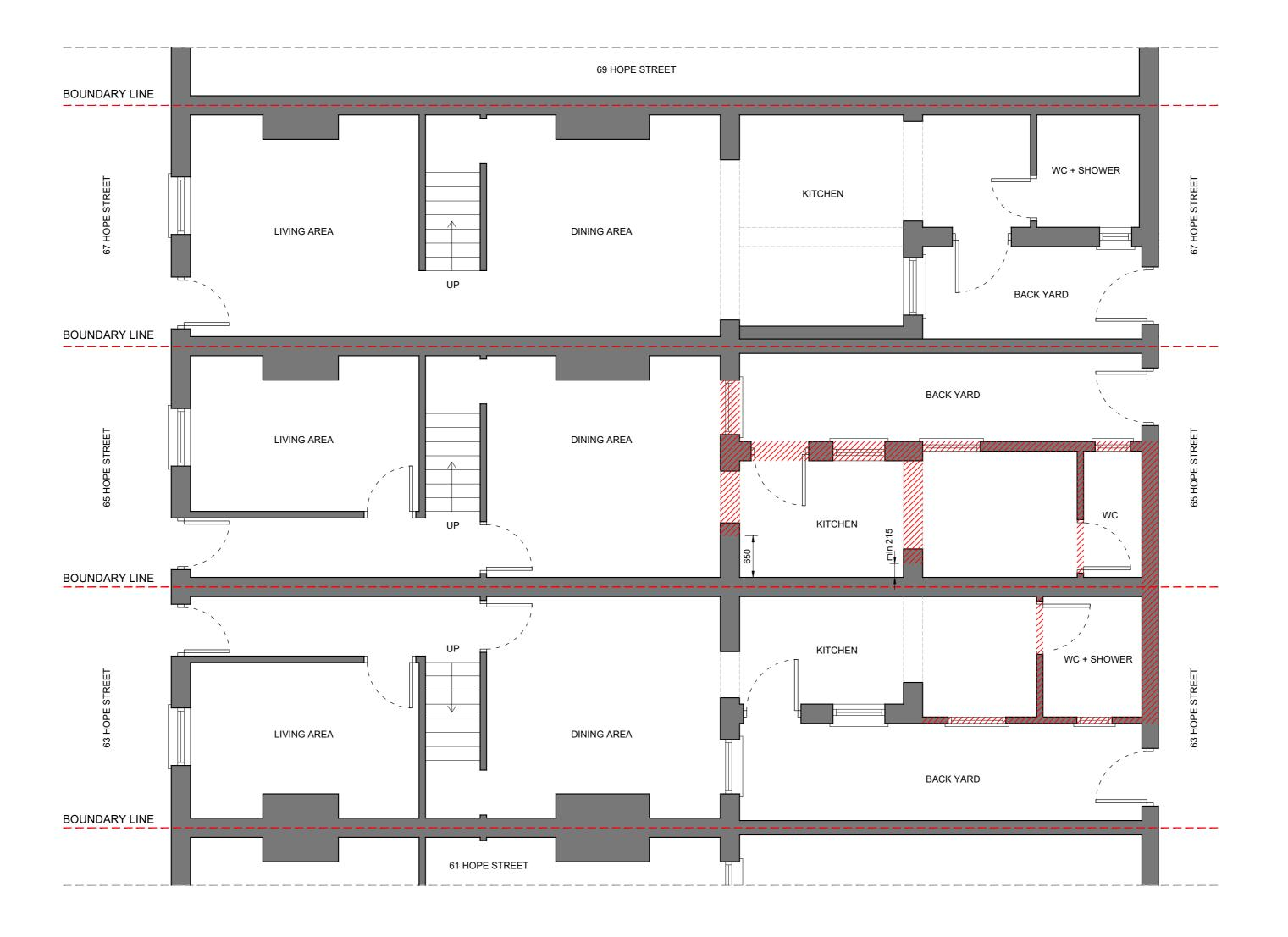
EXISTING GROUND FLOOR PLAN + DEMOLITIONS
